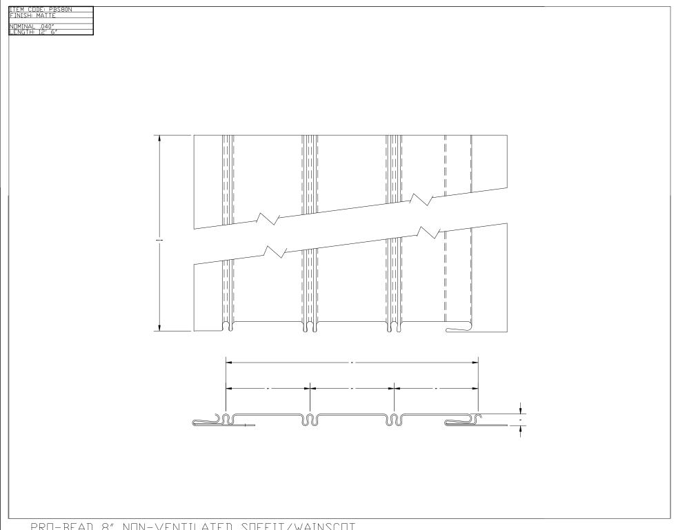
PRO-BEAD 8" NON-VENTILATED SOFFIT/WAINSCOT SCALE:1"=2"
