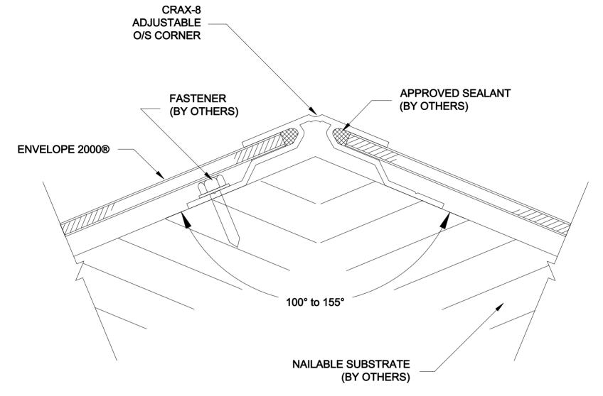
NOTE: FOR NON-NAILABLE SUBSTRATES, FASTENERS MUST BE USED ONLY AT STUD FRAMEWORK LOCATIONS.
