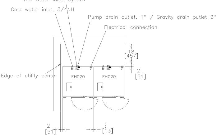
This machine should be installed on an 8" elevated steel base
