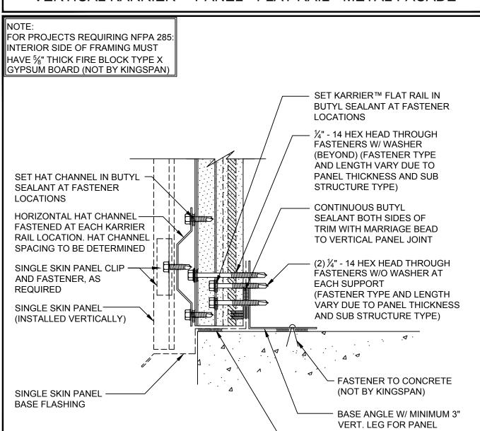
BASE ANGLE W/ MINIMUM 3" VERT. LEG FOR PANEL ATTACHMENT SET IN SEALANT (NOT BY KINGSPAN)
