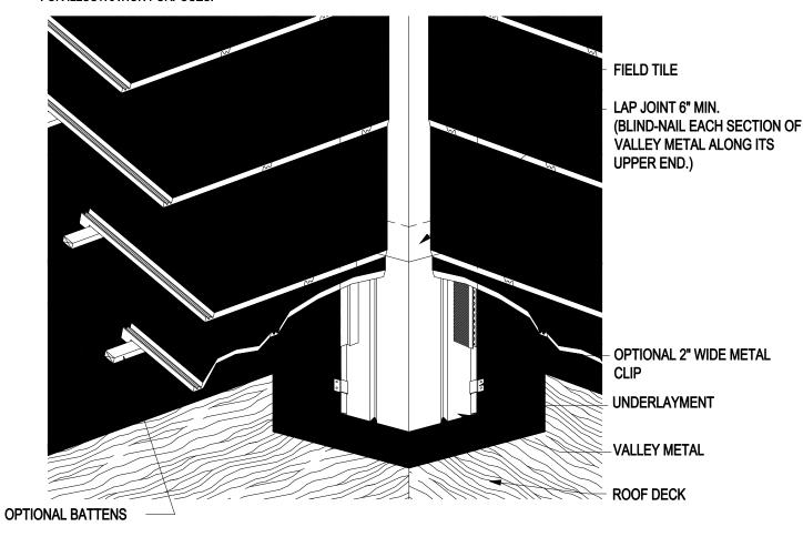
Note: Tile valleys may be cut closed or open. Valley metals shall conform to IBC section 1507.3.9, IRC R905.3.8 and UBC section 1508.4. When flat profiled tile is installed as "closed valley" a ribbed valley metal or a single crown valley metal with a batten extension shall be used.
