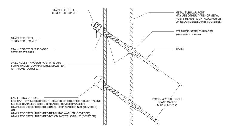
(NOTE: TERMINATION DETAIL SIMILAR FOR WOOD POSTS, BUT TERMINALS MAY REQUIRE A FLAT WASHER BEHIND THE BEVELED WASHER TO PROVIDE ADDITIONAL BEARING SURFACE).
