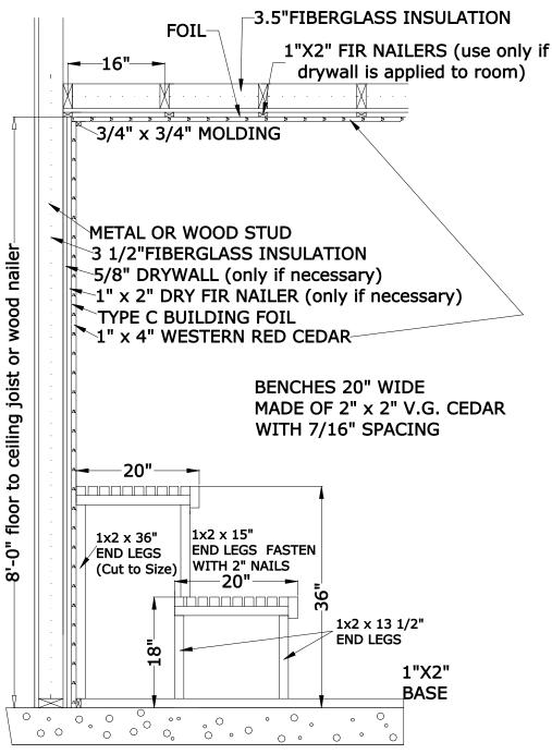
Sauna paneling may be fastened directly to the wooden stud frame. If metal framing is used, 5/8" sheetrock should be added to frame and then 3/4" thick wooden naiing strips should be added over the sheetrock.
