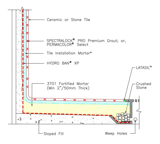
\* Tile installation mortar to be 254 Platinum, 257 TITANIUM<sup>™</sup> or MULTIMAX<sup>™</sup> LITE. Turn waterproofinh membrane up 3" (76mm) above curb of flood point.
