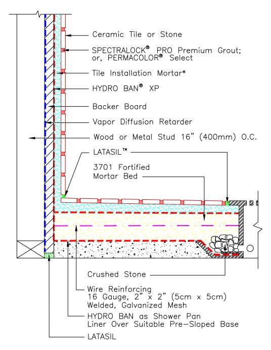
\* Tile installation mortar to be either 254 Platinum, 257 TITANIUM $^{\text{TM}}$  or MULTIMAX $^{\text{TM}}$  LITE. Vapor diffusion retarder use, type and location to be determined by project design professional.
