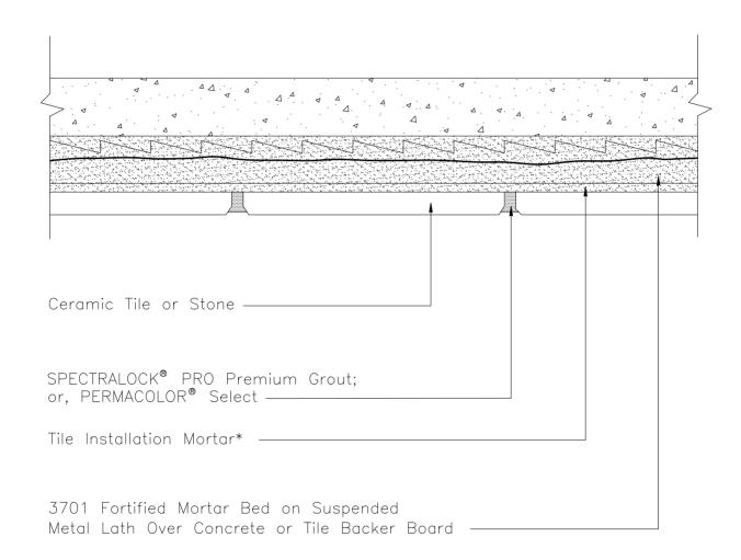
\* Tile installation mortar to be either 254 Platinum, 257 TITANIUM™ or MULTIMAX™ LITE.
