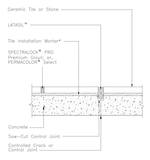
\* Tile installation mortar to be either 254 Platinum, 257 TITANIUM™ or MULTIMAX™ LITE.
