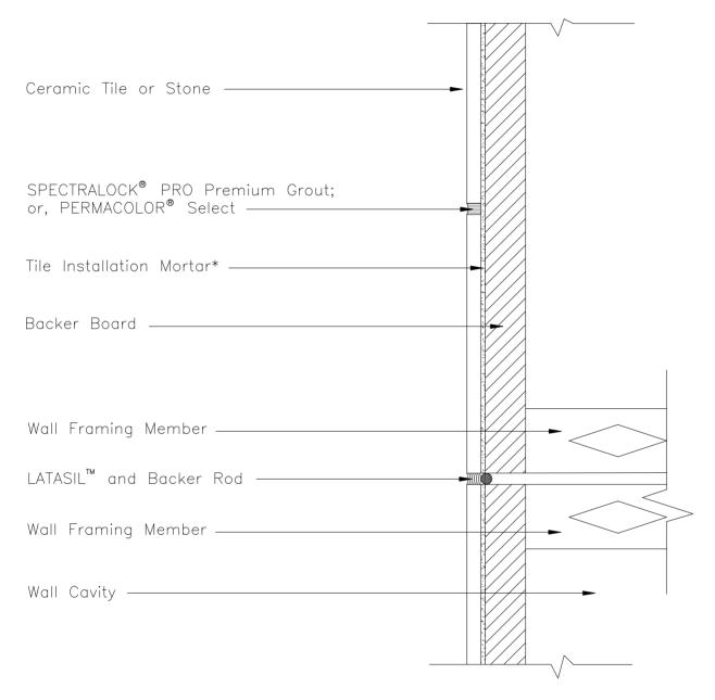
\* Tile installation mortar to be either 254 Platinum, 257 TITANIUM™ or MULTIMAX™ LITE.
