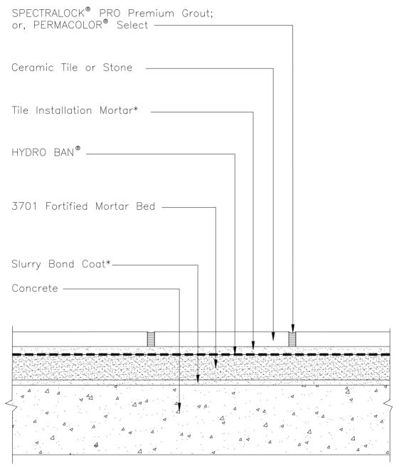
\* Tile installation mortar to be either 254 Platinum, 257 TITANIUM<sup>™</sup> or MULTIMAX<sup>™</sup> LITE.
