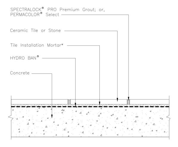
\* Tile installation mortar to be either 254 Platinum, 257 TITANIUM™ or MULTIMAX™ LITE.
