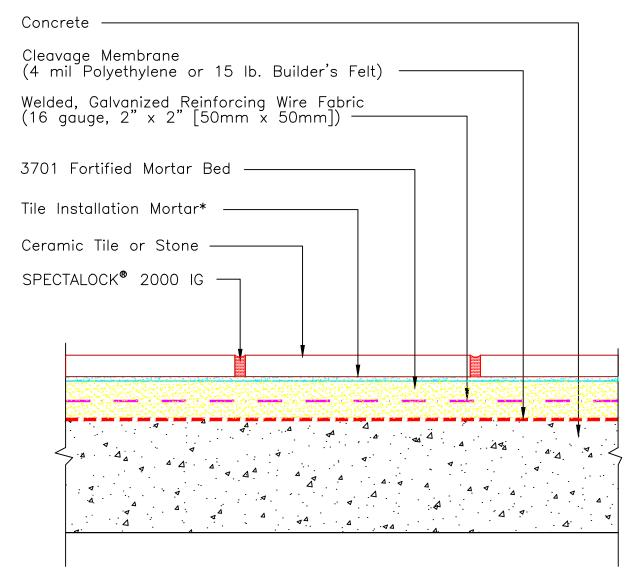
\* Tile installation mortar to be either 254 Platinum, 257 TITANIUM™ or MULTIMAX™ LITE.
