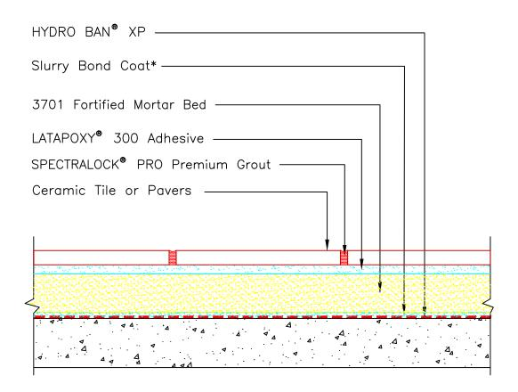
\* Slurry bond coat to be either 254 Platinum, 257 TITANIUM™ or MULTIMAX™ LITE.
