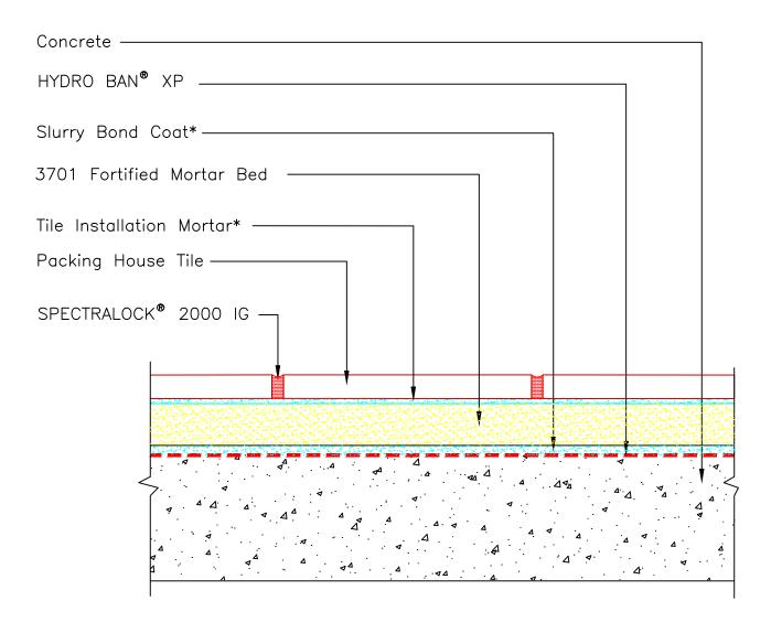
\* Slurry bond coat and tile installation mortar to be either 254 Platinum, 257 TITANIUM™ or MULTIMAX™ LITE.
