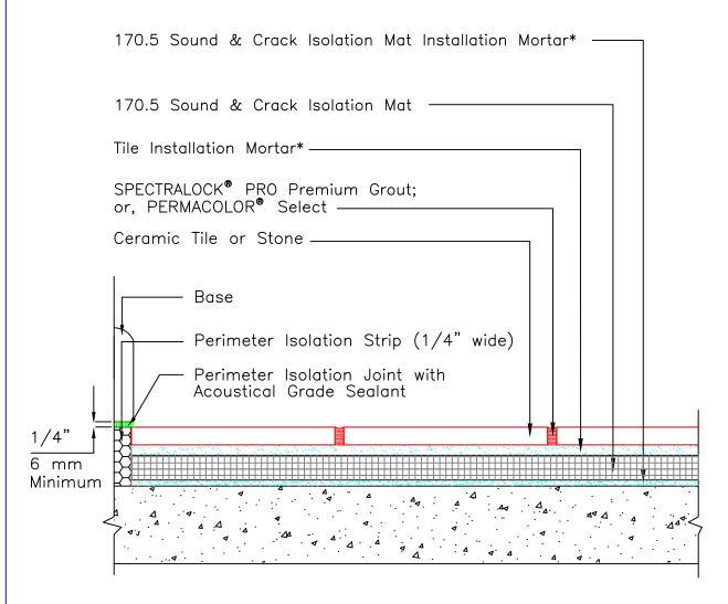
\* 170.5 Sound & Crack Isolation Mat installation mortar and tile installation mortar to be either 254 Platinum, 257 TITANIUM™ or MULTIMAX™ LITE.
