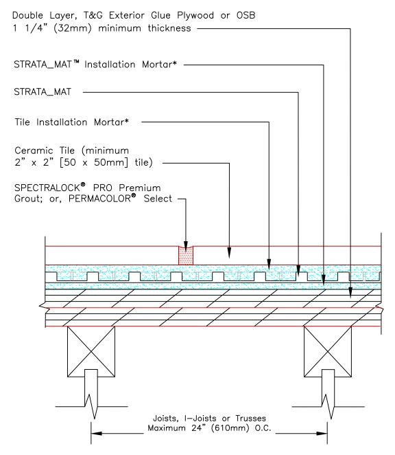
\* STRATA\_MAT installation mortar and tile installation mortar to be either 254 Platinum, 257 TITANIUM™ or MULTIMAX™ LITE.
