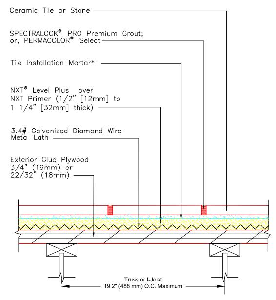
\* Tile installation mortar to be either 254 Platinum, 257 TITANIUM™ or MULTIMAX™ LITE.
