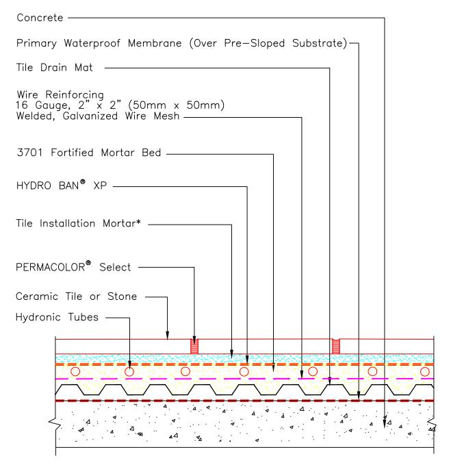
\* Tile installation mortar to be either 254 Platinum, 257 TITANIUM  $^{\text{\tiny M}}$  or MULTIMAX LITE. Install mortar bed to a minimum of  $\frac{1}{2}$ " (12.7mm) above top of radiant heat tubes.
