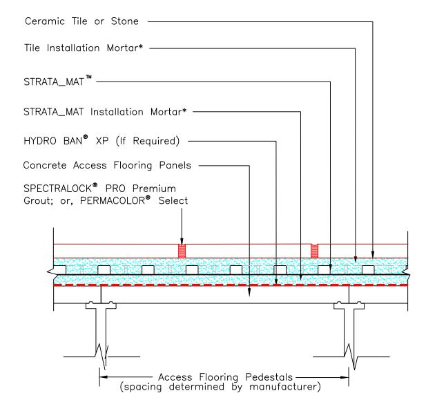
\* STRATA\_MAT installation mortar and tile installation mortar to be either 254 Platinum, 257 TITANIUM™ or MULTIMAX™ LITE.
