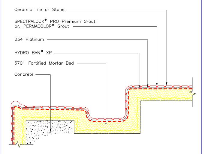
\* Slurry bond coat of 254 Platinum or 257 TITANIUM™ is required under the mortar bed at all horizontal surfaces.
