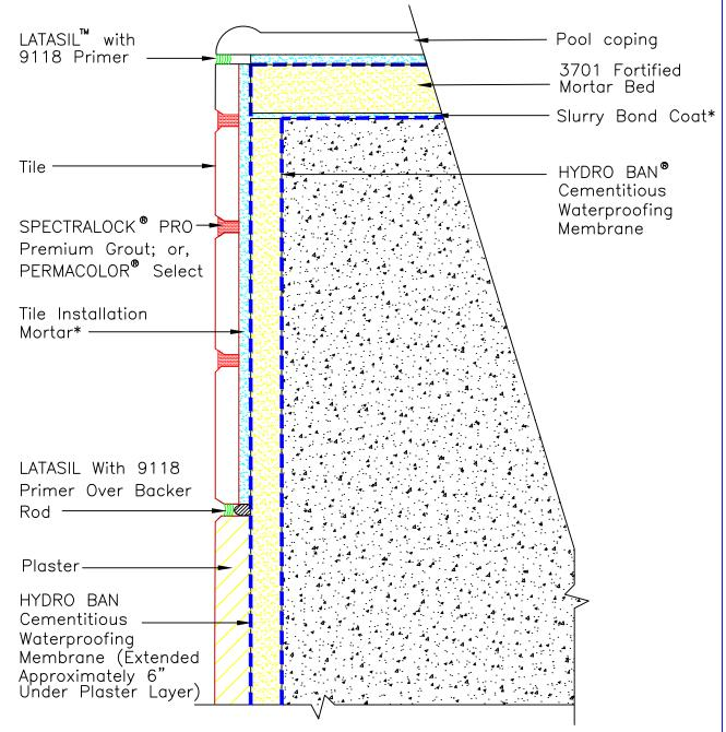
NOTE: Consult with pool plaster manufacturer for bond coat requirements under their material. \* Slurry Bond Coat and Tile Installation Mortar to be 254 Platinum, 257 TITANIUM™ or MULTIMAX™ LITE.
