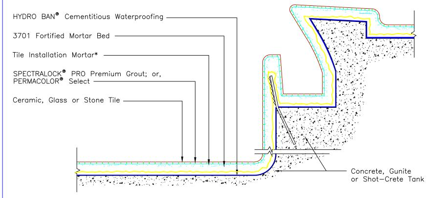
\* Slurry bond coat is required under the mortar bed at all horizontal surfaces. Slurry bond coat and tile installation mortar to be either 254 Platinum, 257 TITANIUM™ or MULTIMAX™ LITE. Movement joints are required at all changes of plane, around all penetrations, and throughout field on floors and walls. Use LATICRETE LATASIL with LATICRETE 9118 Primer in movement joints. Refer to TCNA EJ−171 for more information on movement joints.
