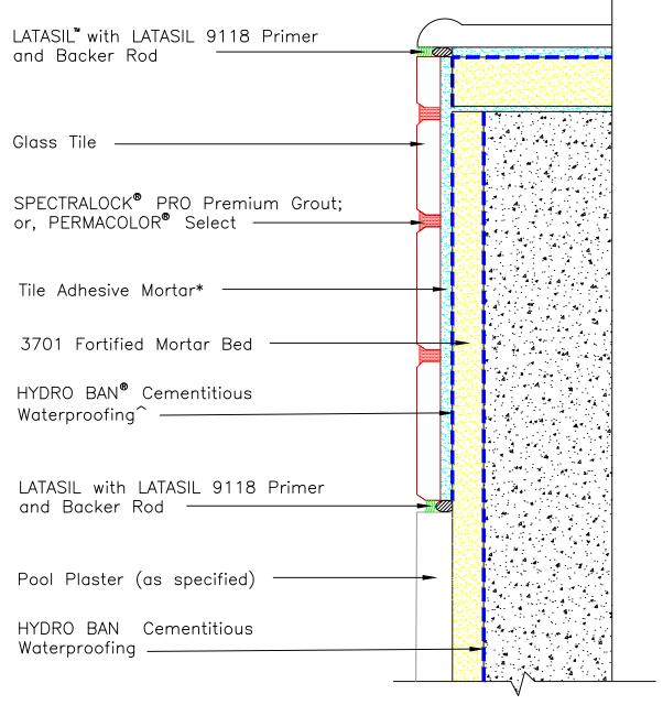
NOTE: Consult with pool plaster manufacturer on bond coat requirements under their material. \* Tile Adhesive Mortar to be LATICRETE Glass Tile Adhesive Lite, 254 Platinum (White), 257 TITANIUM™ (White) or MULTIMAX™ LITE (White). ^ Check with glass tile manufacturer for requirement of cementitious waterproofing directly under their tile to prevent "ghosting".
