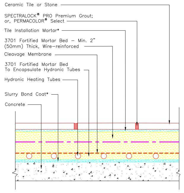
Slurry bond coat and tile installation mortar to be either 254 Platinum, 257 TITANIUM<sup>™</sup> or MULTIMAX<sup>™</sup> LITE. Thickness of mortar bed encapsulating hydronic tubes should be brought just to top of hydronic tubes.
