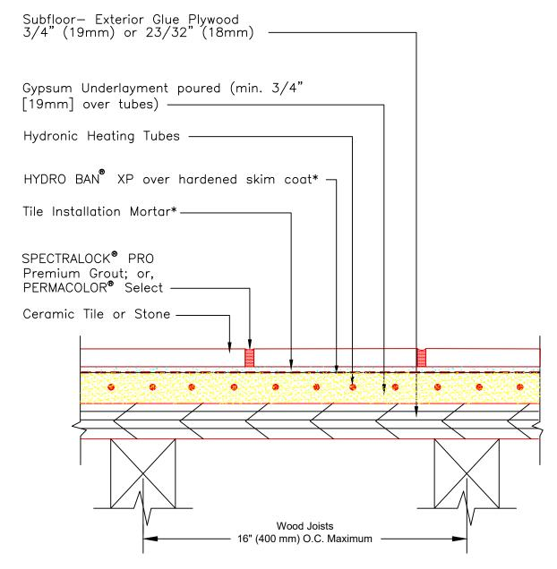
\* Skim coat and tile installation mortar to be either 254 Platinum, 257 TITANIUM™ or MULTIMAX™ LITE.
