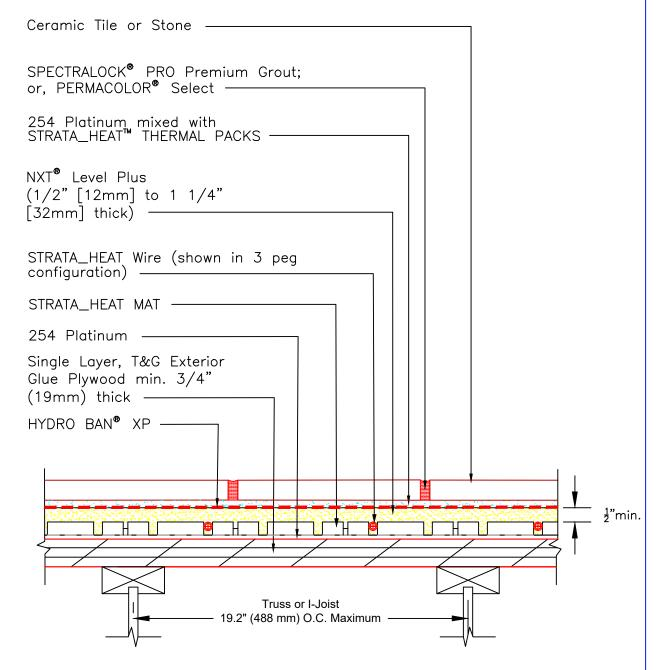
NOTE: NXT Level Plus to be sufficiently dry prior to application of HYDRO BAN XP.
