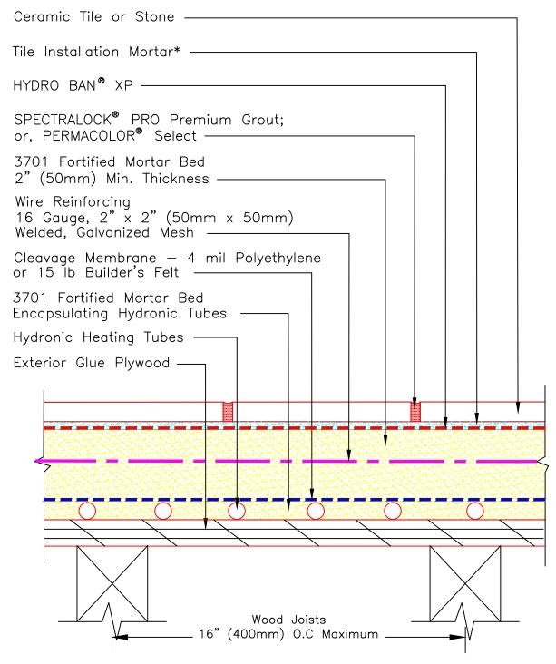
\* Tile installation mortar to be either 254 Platinum, 257 TITANIUM™ or MULTIMAX™ LITE.
