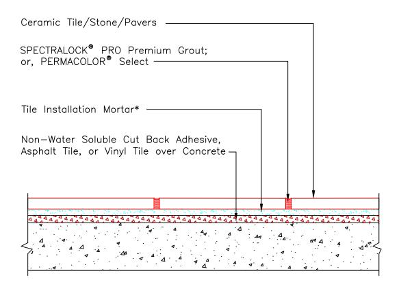
\* Tile installation mortar to be either LATAPOXY<sup>®</sup> 300 Adhesive, 254 Platinum, 257 TITANIUM<sup>™</sup> or MULTIMAX<sup>™</sup> LITE.
