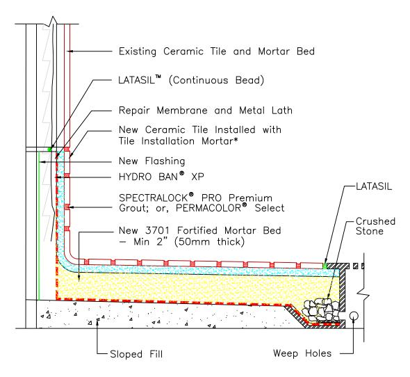
\* Turn waterproofing membrane up at least 3" (76mm) above curb or flood point. Tile installation mortar to be either 254 Platinum, 257 TITANIUM™ or MULTIMAX™ LITE.
