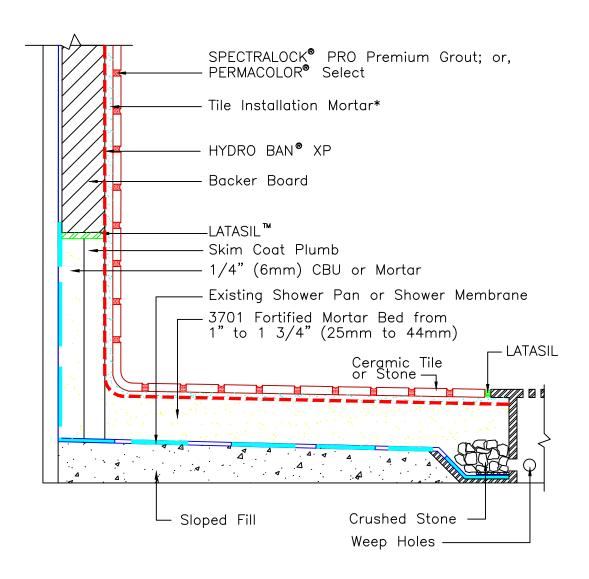
\* Turn waterproofing membrane up at least 3" (76mm) above curb or flood point. Tile installation mortar to be either 254 Platinum, 257 TITANIUM™ or MULTIMAX™ LITE.
