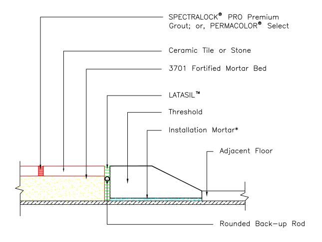
\* Installation mortar to be either 254 Platinum, 257 TITANIUM or™ MULTIMAX™ LITE.
