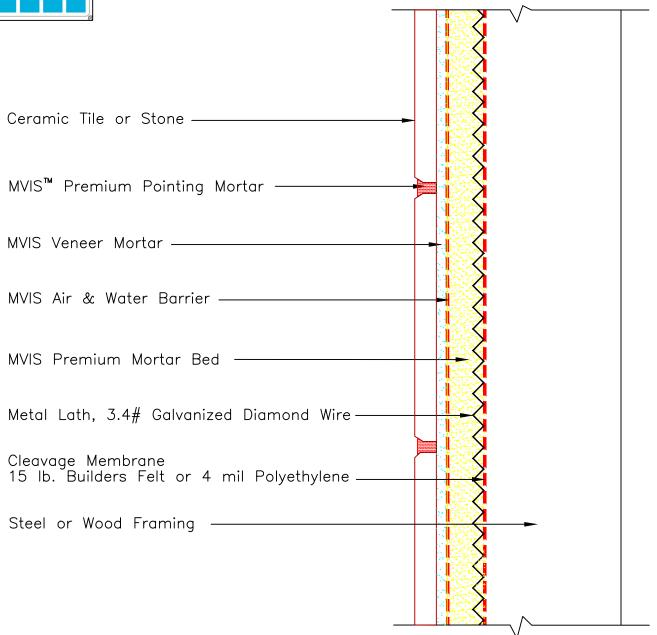
NOTE: Vapor Barrier, Weather Barrier, Separation Sheet, Insulation, Waterproofing, and Furring Type/Location to be Determined by Design Professional. Maximum Allowable Deflection Under All Live, Dead and Impact Loads, Including Concentrated Loads, Must Not Exceed L/600 Where L=Span Length. Design Professional to Ensure Compliance With Building Code(s).
