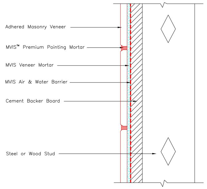
This detail is intended for use in showing installation of LATICRETE products, and should not be used as the design for wall construction. Wall construction system must be designed and approved by project design professional. Wall construction to meet minimum deflection rating of L/600 under anticipated loads. Proper flashing to be installed at top and bottom of wall and any penetrations to prevent water intrusion into wall cavity.
