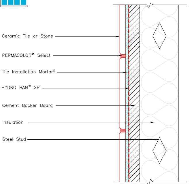
NOTE: Vapor Barrier, Weather Barrier, Separation Sheet, Insulation, Waterproofing, and Furring Type/Location to be Determined by Design Professional. Maximum Allowable Deflection Under All Live, Dead and Impact Loads, Including Concentrated Loads, Must Not Exceed L/600 Where L=Span Length. Design Professional to Ensure Compliance With Building Code(s). \* Tile installation mortar to be either 254 Platinum, 257 TITANIUM™ or MULTIMAX™ LITE.
