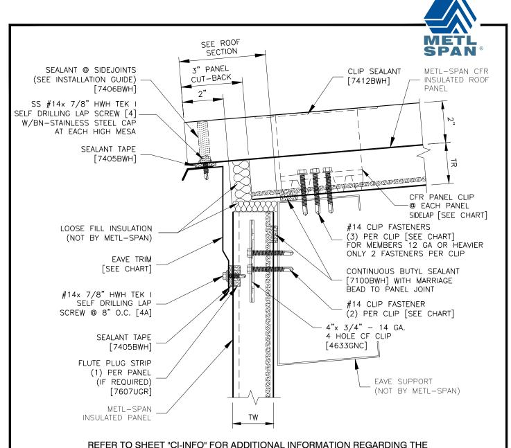
APPLICATION OF SEALANTS, FASTENERS, AND CLOSURE MATERIALS.
