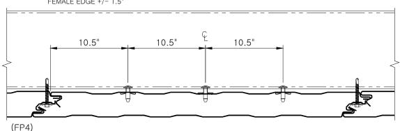
FASTENING PATTERN 4 SIDE JOINT FASTENING WITH THREE DOME HEAD BULB-TITE® RIVETS
