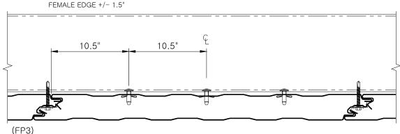
FASTENING PATTERN 3 SIDE JOINT FASTENING AND TWO DOME HEAD BULB-TITE® RIVETS
