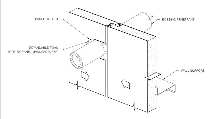
SEE DETAIL CI-CF-PEN-4 FOR SEALANT LOCATIONS SEE DETAIL CI-CF-PEN-5 FOR FLASHING INFORMATION
