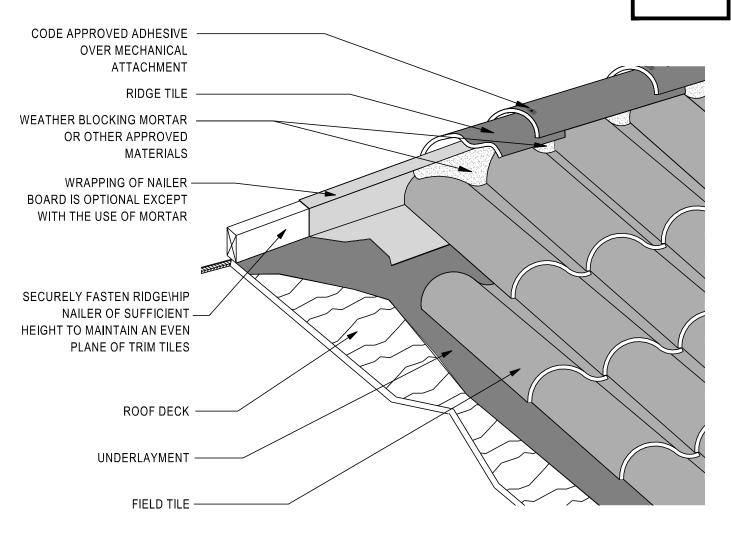
Openings at hips, ridges and head walls including chimneys, skylights, solar panels, and downslope horizontal abutments shall be fitted with weather blocking material to keep water on the surface of the field tile. Other methods approved by local building official will be allowed.
