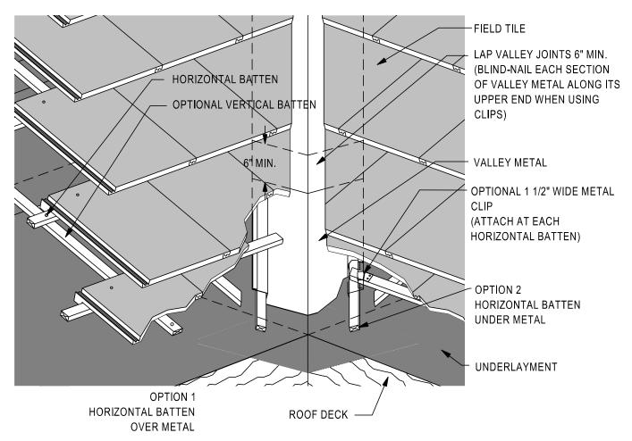
Note: Valley metal shall extend at least 11" from center line each way and shall have a splash diverter rib not less than 1" high at the flow line formed as part of the flashing. Other designs that will handle anticipated water flows may be used upon submission of supporting data indicating that anticipated water flows are equivalent to the code requirements.
