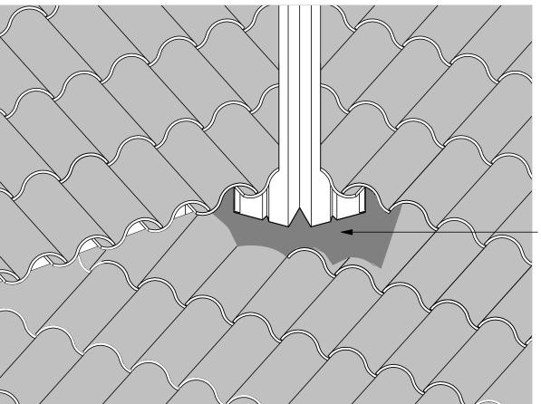
THE VALLEY METAL MUST LAP ONTO THE TILE OF THE COURSE BELOW THE ROOF TRANSITION FLASHING
