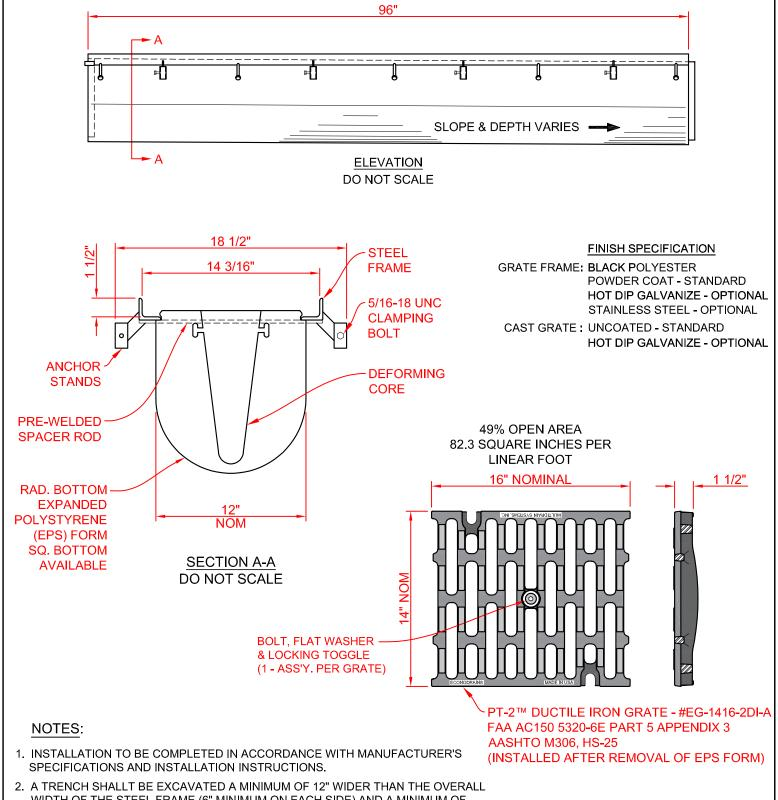
WIDTH OF THE STEEL FRAME (6" MINIMUM ON EACH SIDE) AND A MINIMUM OF 6 INCHES DEEPER THAN THE OVERALL DEPTH OF THE ECONODRAIN EPS FORM.
