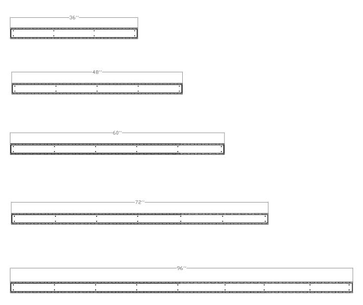
BASE LENGTH COULD BE REDUCED AND COVER BE ADJUSTED TO THE DESIRED LENGTH.
