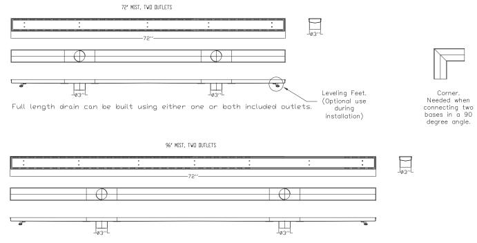
Full length drain can be built using either one or both included outlets.
