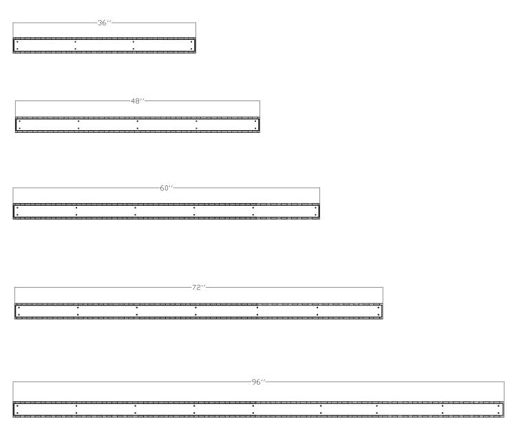
BASE LENGTH COULD BE REDUCED AND COVER BE ADJUSTED TO THE DESIRED LENGTH.
