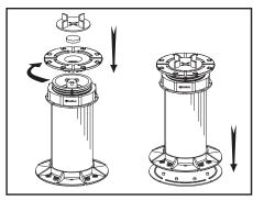
5. Complete assemble by rotating and aligning Uni-Cap<sup>TM</sup> with Uni-Insert<sup>TM</sup> and Lock Ring. Align & attach Buffer Pad to Uni-Base<sup>TM</sup>.
