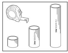
2. Using a laser, determine final height of pedestals. Deduct ½" for base & cap assembly. Measure & mark PVC pipe to be cut.
