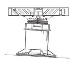
8. Use a spirit level to level Uni-Cap<sup>TM</sup> in any direction.
