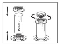
4. Assemble by inserting cut PVC pipe in to Uni-Base<sup>™</sup> and Uni-Collar<sup>™</sup> in to other end of PVC pipe. Screw Uni-Insert<sup>™</sup> in to Uni-Collar<sup>™</sup> minimum of 2 threads.
