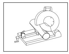
3. Cut PVC pipe to required height with a 12" chop saw. Using sand paper, remove any burrs from cut ends.
