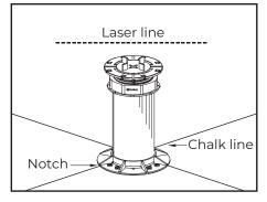
6. Position pedestal under laser line and align Buffer Pad notch with chalk line.
