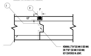
REINFORCING CONTINUOUS THROUGH JOINT.
