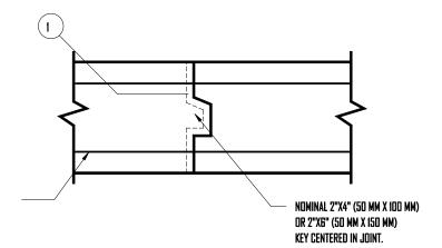
REINFORCING CONTINUOUS THROUGH JOINT.
