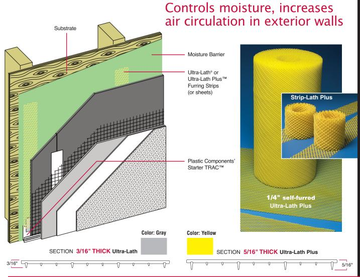
Plastic Components' **Ultra-Lath® plastic lath** is ideal for all vertical cladding with drainage.
